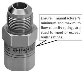
Figure 45 - Excess Flow Valve (EFV)
