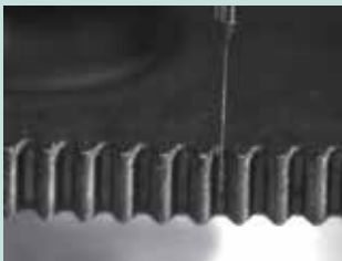
Measuring form of micro gear teeth
