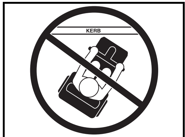
Figure 4. Incorrect Kerb Approach
