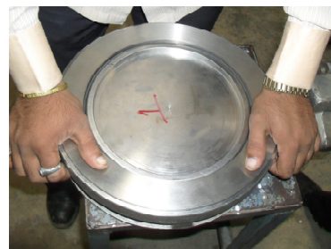
Fig 5.3:Fixing the seat and seat retainer assembly in to the body
