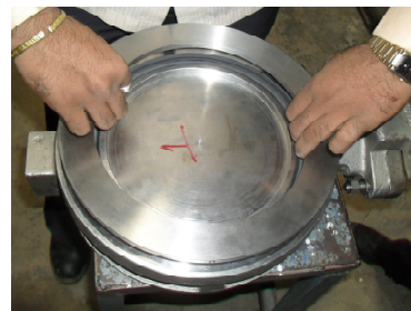
Fig 5.2:Installing seat and seat retainer assembly
