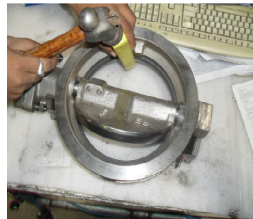
Fig 5.1:Way to remove seat retainer
