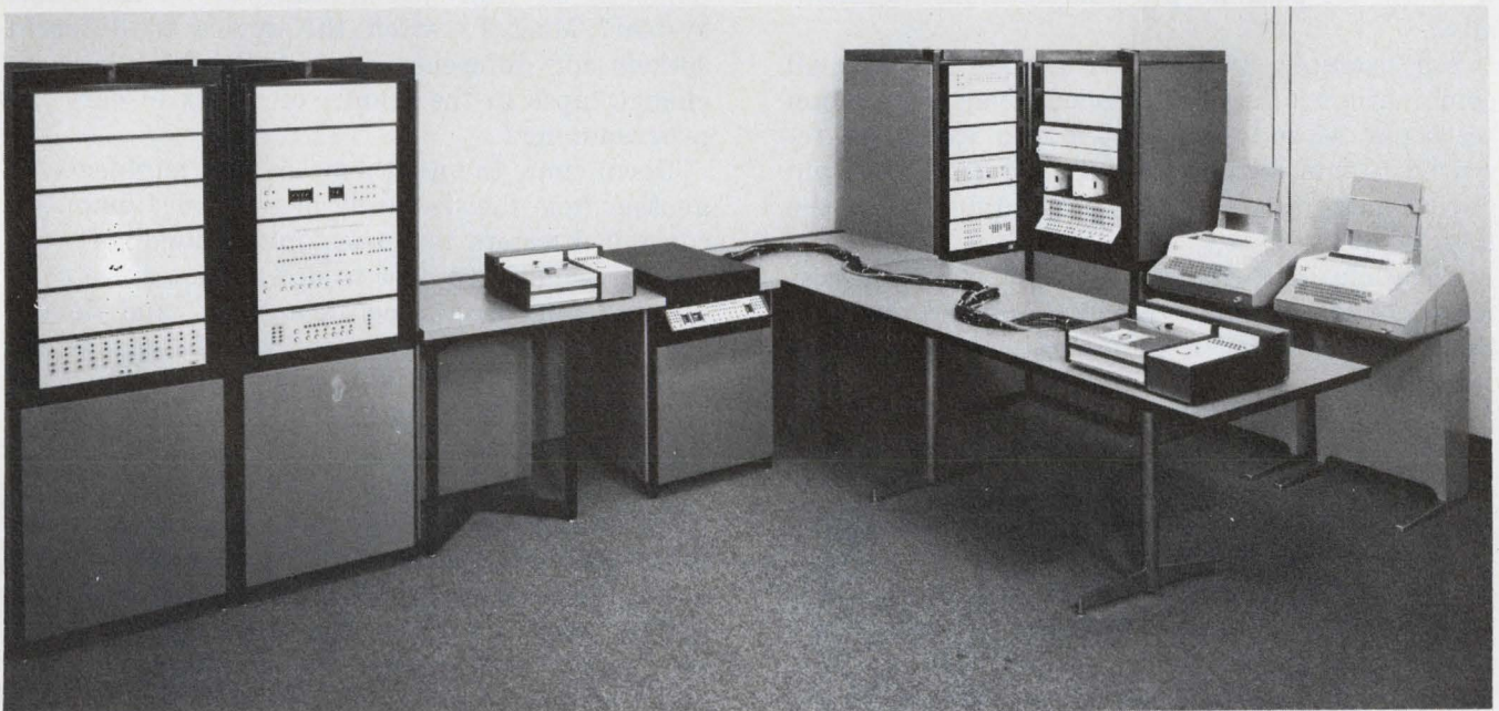
Representative of the production-oriented large-scale test systems is the J277 computerized MOS system, manufactured by Teradyne. Its features include multiplexed
