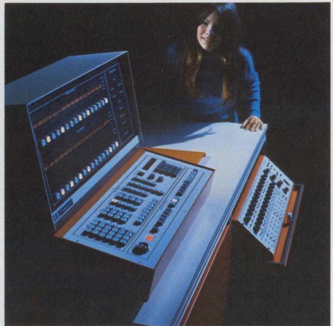
Semiconductor Test Systems' Venture II , a dedicated semiconductor-memory tester, has a microprogrammed controller and an English-language entry console.
