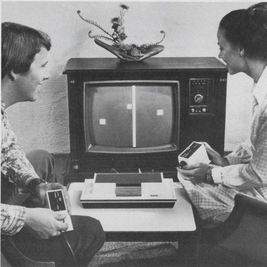
An electronic game simulator that connects to the TV set antenna, by the Magnavox Co., permits TV viewers to play a dozen games of skill or chance. Figures on the screen are manipulated by the contestants.
