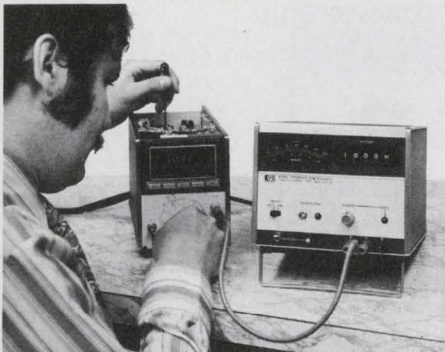
A 6115A precision power supply is used to calibrate the dc voltmeter section of an HP multimeter.
