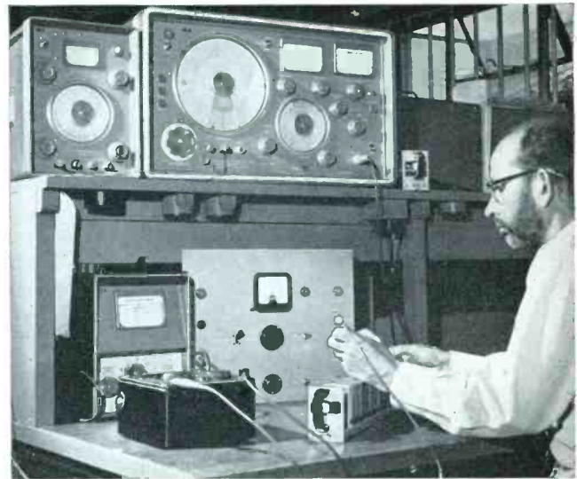
Setting up I.L.S. equipment in the Marconi test room at London Airport. The crystal oscillator output of the TF 801D/5M1 modulated to 90% by the R-C Oscillator type TF 1101 provides a test signal for a 75 Mc/s marker receiver
