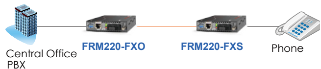
Figure 2 : Voice Transmission from 2km to 120km over fiber
