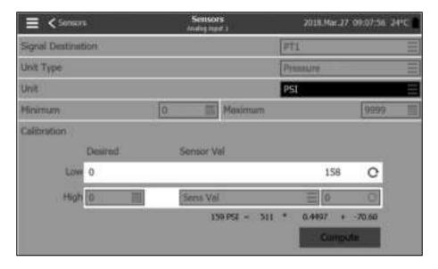
For the pressure transducer PT1, the low point (zero) is automatically acquired during first power up. It can be reacquired by pressing the blue round arrow. The high point needs to be entered in order to calibrate the sensor.
