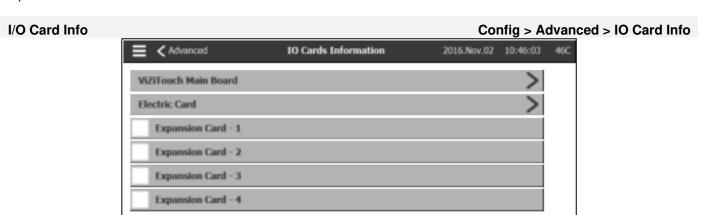
This page is used to visualize the ViZitouch and the IO Card registers by pressing on the blue arrows on the right of the screen. Expansion Cards can also be installed via this page.
