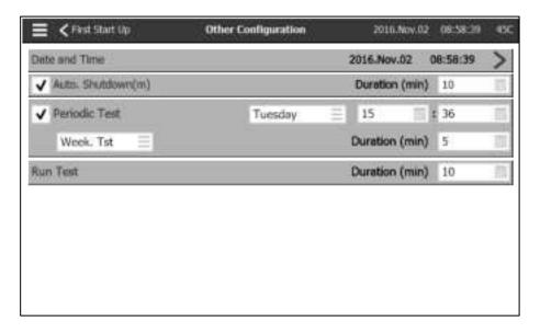
Go back to the controller start-up page and press the "Other Configuration" button. Enter the time and date. Select the "Automatic shutdown" and the duration the pump will keep running after the automatic stop if an automatic stop is desired. Select the frequency at which the periodic test will occur, the day of the week, the hour and the duration of the test. Also, enter the duration of the Manual Run Test.
