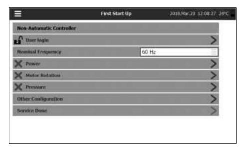
Once the controller has booted up, the "First Start Up" page appears. The controller will automatically detect and display the frequency of the power source. It is then possible to manually choose the frequency of the voltage. Press "User Login" and enter a valid authorization code. Once logged in, press "Power".
