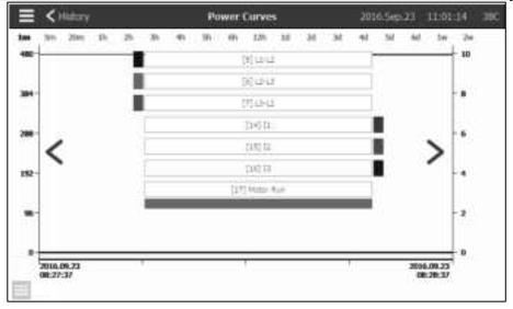
On this page, a graphic of the 3 line voltages, the 3 line currents and the motor running through time can be viewed. By pressing on the screen, the caption will disappear or will be displayed. The time scale can be changed by pressing the time span desired on top of the screen (from 1 minute to 2 weeks). The blue arrows on both sides of the graphic are used to navigate through time. The blue button in the bottom left corner leads to the table used to generate this graph.
