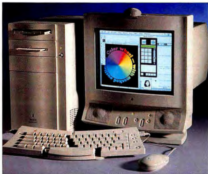
With Apple's AudioVision monitor and a built-in DSP, the Quadra 840AV is ready to handle voice data.
