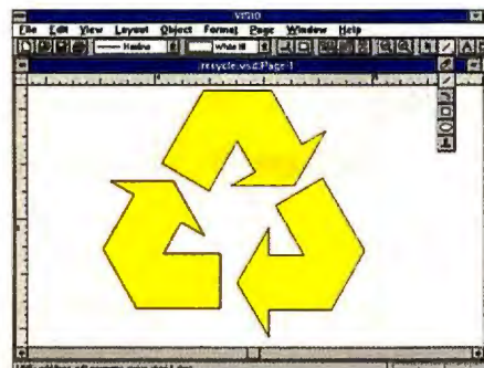
This recycling symbol was created in Visio 2.0 in about 20 minutes. The predrawn arrows were modified using the line tool and fragment command and then rotated using the rotation tool. The program's grid helped in aligning the arrows.
