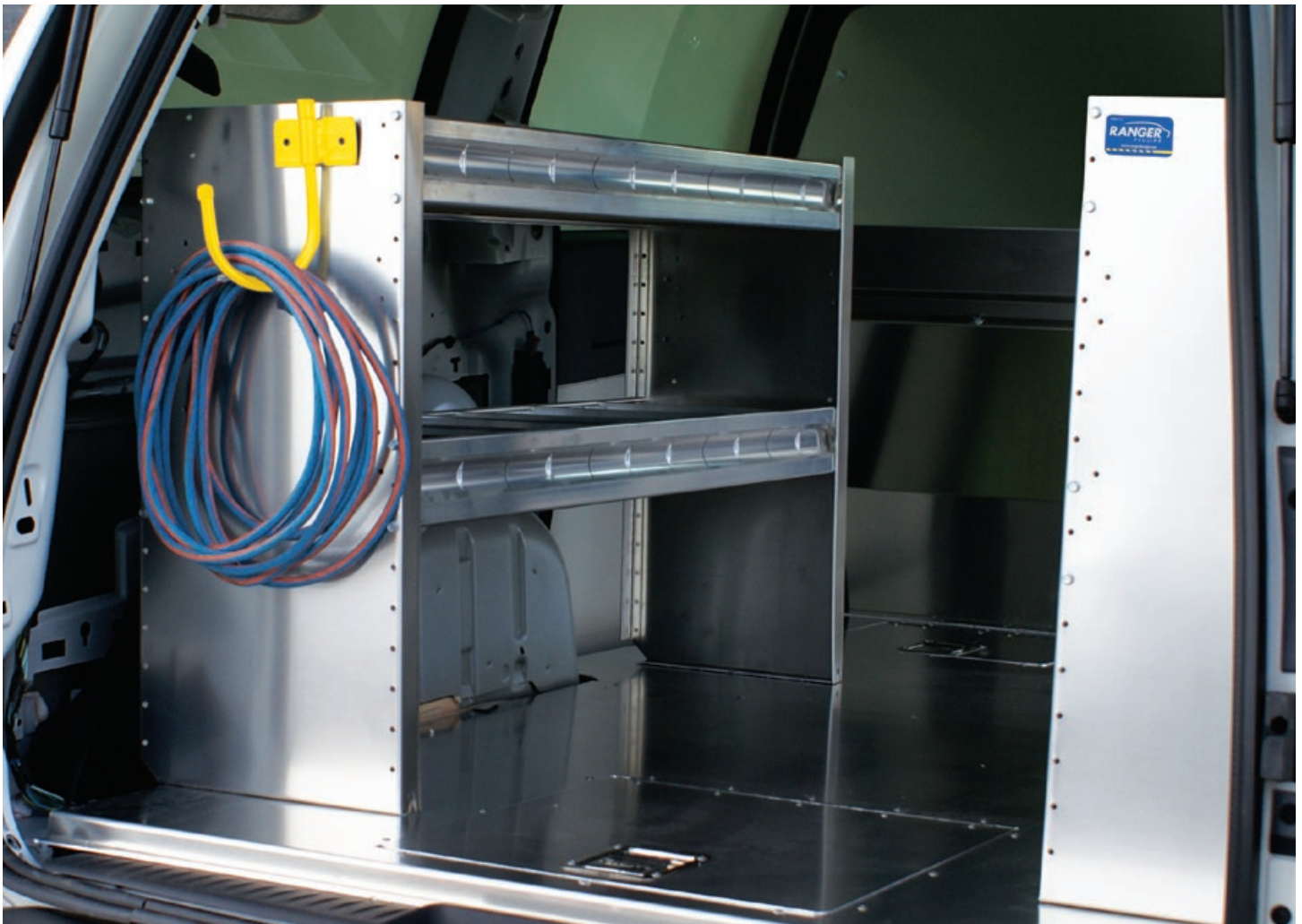
Model # 3010-DC = Drill free installation
