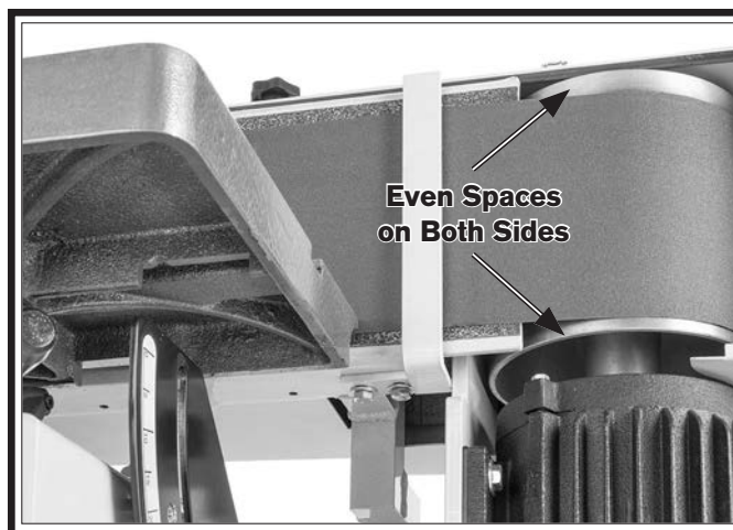
Figure 41. Example of sanding belt centered on drive roller.
