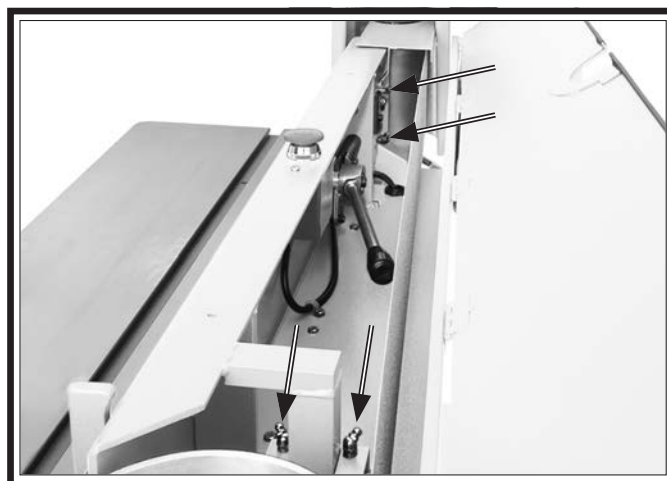
Figure 75. Location of grease fittings inside sanding body.
