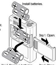
Step 2. Remove batteries. Step 6. Close.
