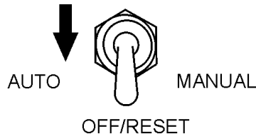
Figure 43. Auto Off/Reset Manual Switch (Off/Reset)
