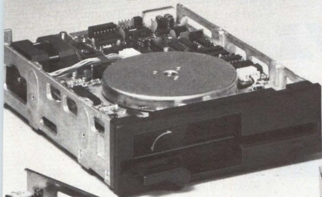
FD-55 Series 5 1/4-Inch Half-High Floppy Disk Drives Capacities from 250 KB - 1.6 MB. 2 new LSI's, 4.9 watts operating power. Brushless DC Direct Drive Motor.
