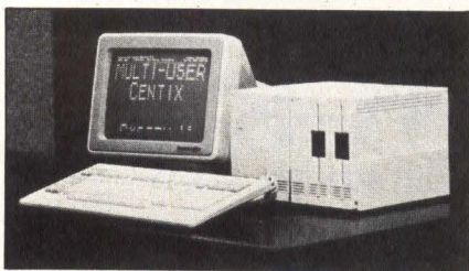
The Burroughs XE 550 is based on the MC68010 processor from Motorola, but includes auxiliary processors based on Intel's 80186.
