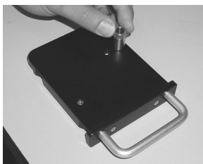
Figure 3: Tightening the lock-ring.
