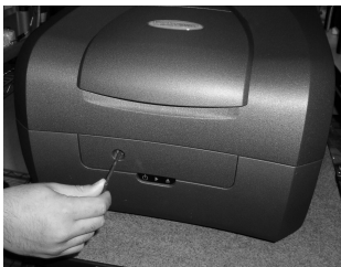
Figure 1: Opening the filter compartment.
