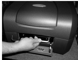
Figure 2: Removing the filter cartridge.
