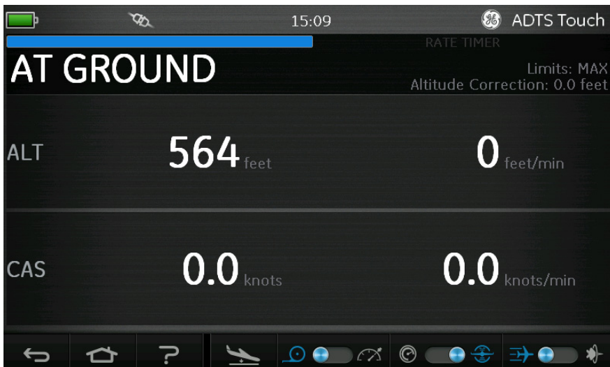
Figure 3-18 Go to ground complete
