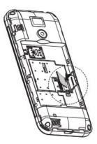
1.5 Insert the the microSD card into the slot with its gold contacts facing down.
