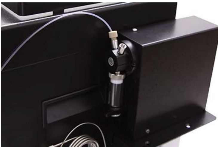
Figure 4-21 Connection of the waste tubing from the EZ Prep inject valve to the left AutoInjector Module port
