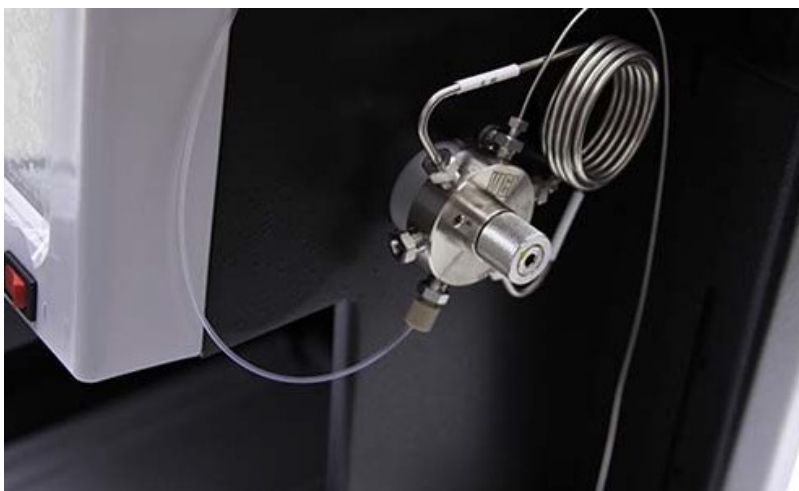
Figure 4-25 Sample tube fitting with the plastic fitting removed
