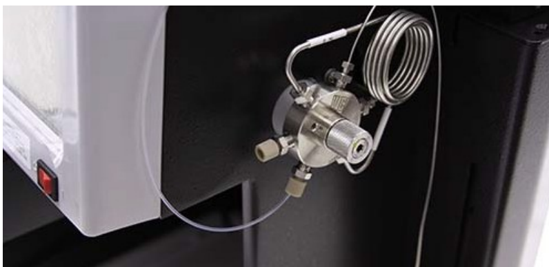
Figure 3-28 Sample probe tube fitting connected to the EZ Prep inject valve
