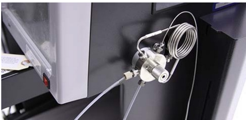
Figure 3-30 Sample probe tube fitting with sample probe tubing attached
