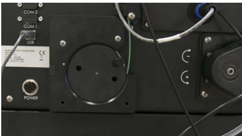
Figure 3-19 AutoSampler Module rotor before after the bottom screws
