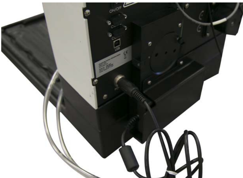
Figure 3-22 AutoSampler Module with power connection made
