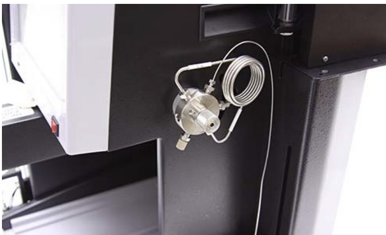
Figure 3-32 Waste tubing fitting attached to the EZ Prep inject valve
