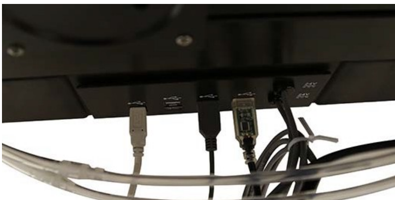
Figure 3-16 AutoSampler Module USB-A connection (center)
