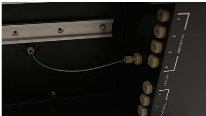
Figure 4-13 Connected Column Selector Module outlet port tubing
