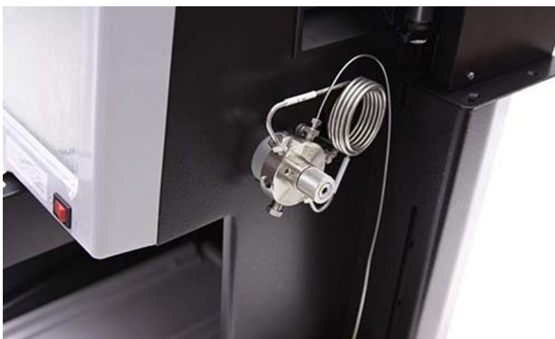
Figure 3-33 Waste fitting with the plastic fitting removed
