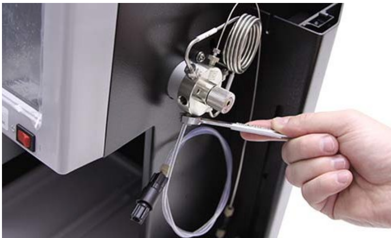
Figure 4-17 Removing the waste line from the EZ Prep inject valve
