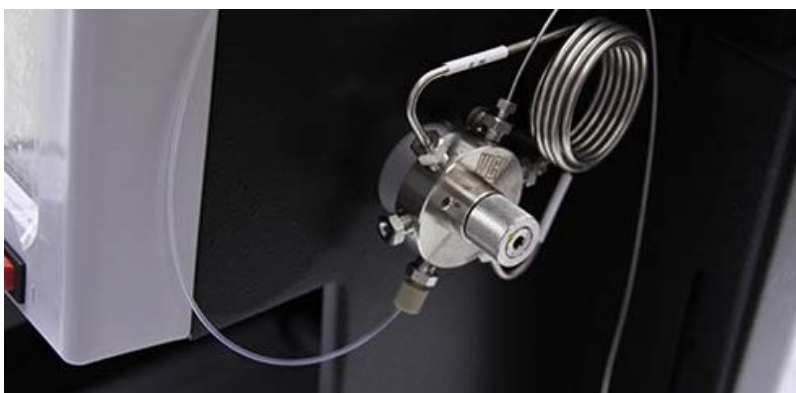
Figure 3-29 Sample probe tube fitting with the plastic fitting removed
