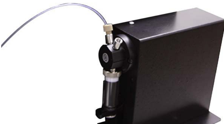
Figure 3-35 Connection of the waste tubing from the EZ Prep inject valve to the left AutoInjector Module port
