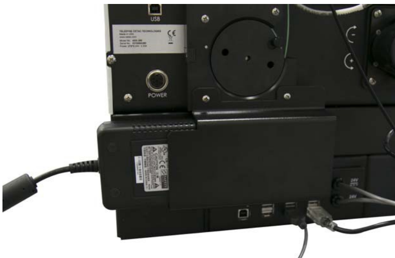
Figure 3-21 Inserting the power supply into the power supply bracket
