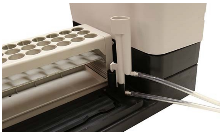
Figure 3-8 AutoSampler Module wash station with tubing attached
