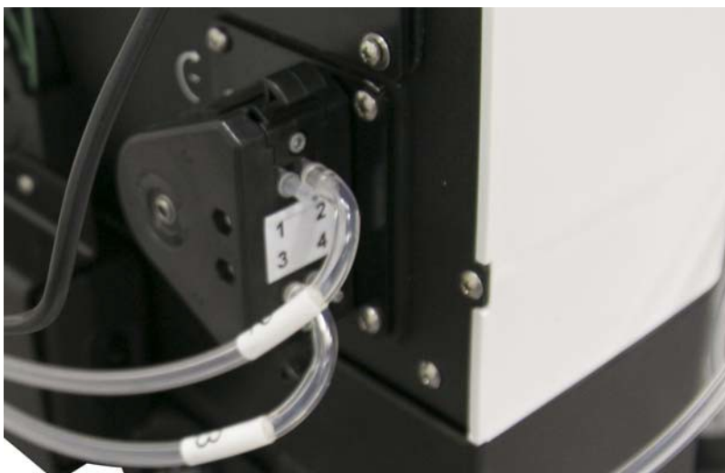
Figure 3-10 Routing the top section of wash station tubing
