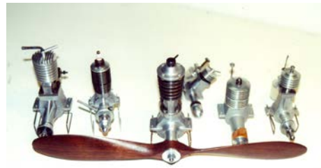
Selection of engines that Bert built. From left: Sparey SCC, M&M 29, Rutch Nova 4 cc, Bulldog Mills, Bulldog 2.5 cc, Deezil replica.
