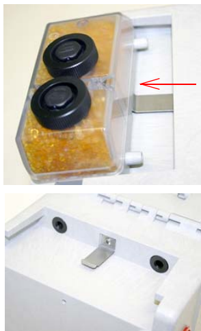
Figure 4-4 Removing the external desiccant cartridge
