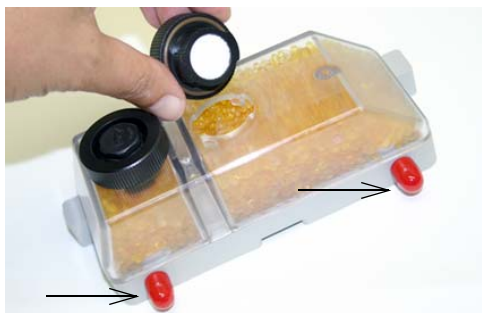
Figure 4-5 Opening the desiccant cartridge chambers
