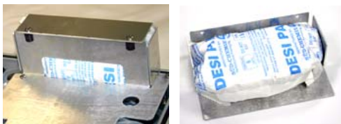
Figure 4-1 Removing the internal desiccant bag
