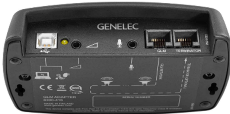
Figure 41. GLM Network Adapter connections from left to right, USB to computer or to USB power supply, hardware level controller input, GLM measurement microphone input, GLM network and terminator connectors.
