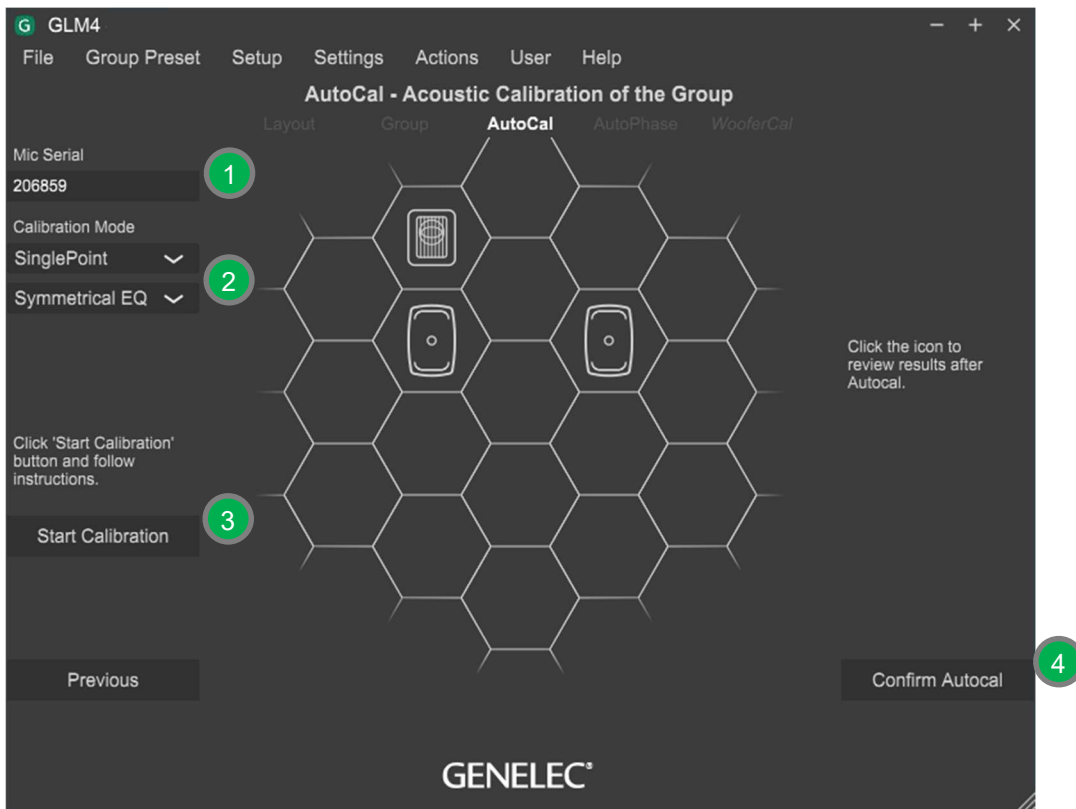
Figure 18. Steps in running the AutoCal automatic system calibration process
