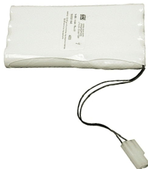
Figure 97. Internal Battery Pack and Connector.
