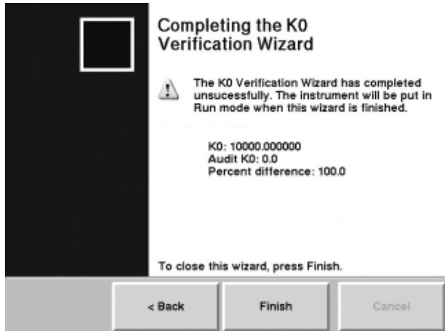
Figure 5-70. Completing the K0 Verification Wizard screen with a fail message.
