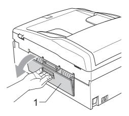
3 Clean the Paper Pick-up Roller (1) with isopropyl alcohol on a cotton swab.
