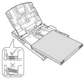
Gently adjust the paper side guides (1) to fit the paper with both hands. Make sure the paper side guides touch the sides of the paper.
