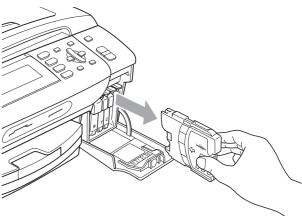
Open the new ink cartridge bag for the color shown on the LCD, and then take out the ink cartridge.
