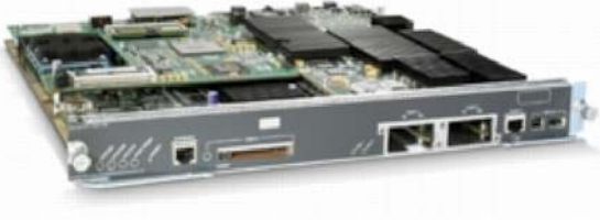
Figure 2. Supervisor Engine 32 with 2-Port 10 Gigabit Ethernet and PFC3B
