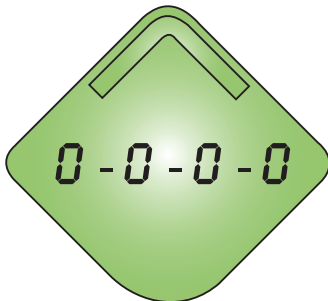
'Squawk' Pattern on the LCD Meter of a Located 2160
