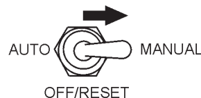
Figure 41. MPEC Control Switch (Manual Position)
