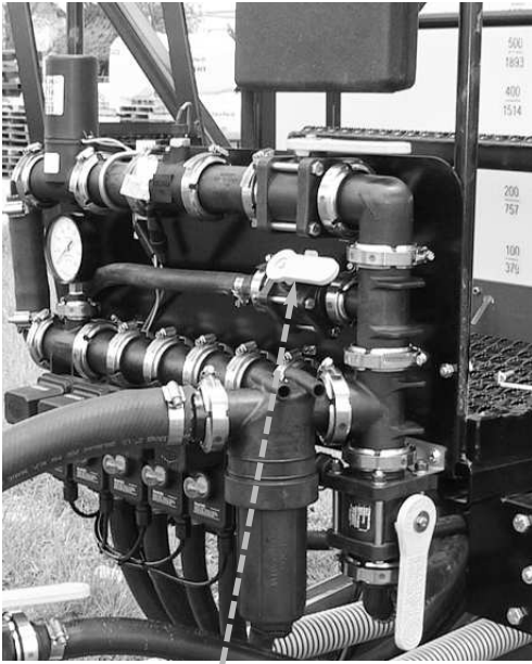
Tank rinse valve, “on” position
