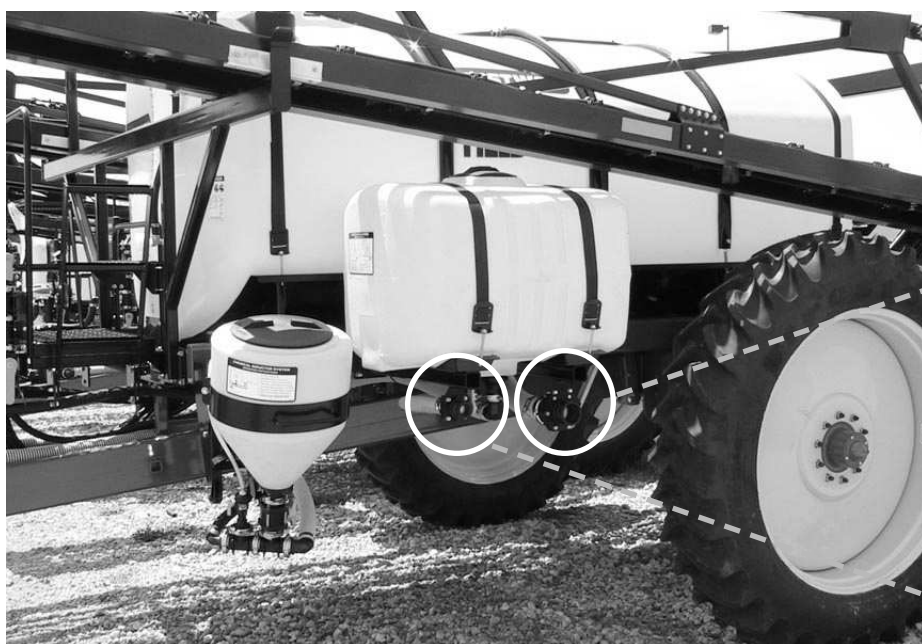
Rinse tank Quick-Fill, “off” position
