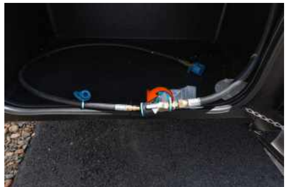
Figure 40.2 Propane Quick Connect With Valve Lock in Closed Position
