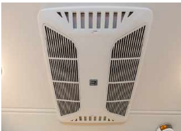
Figure 34.1 Roof Mount A/C with Chill Grill Vents
