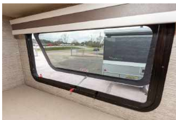
Figure 28.4 Push Arm Outward to Lock Emergency Window in Place. Remove Screens Prior to Exiting.
