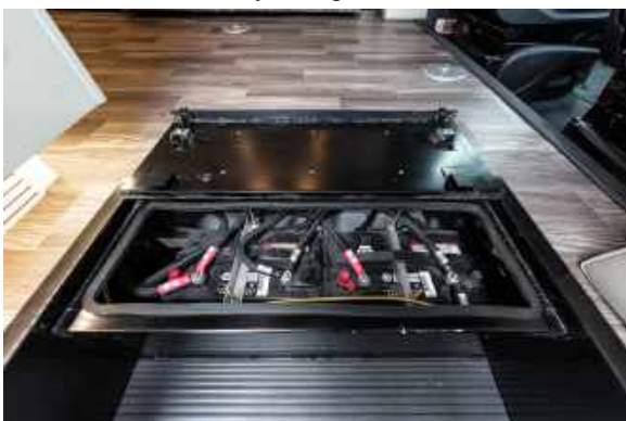
Figure 76.3 Battery Compartment Unlocked to Access Battery Distribution Center
