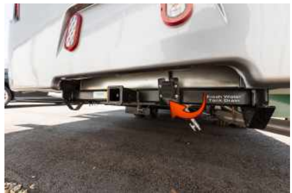
Figure 85.1 7 Pin Connector on Tow Hitch
