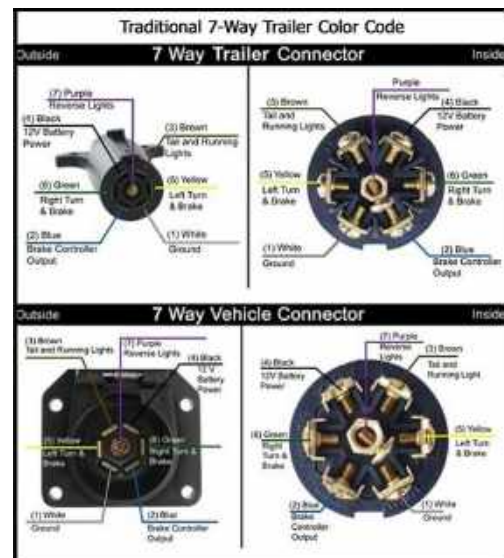
Figure 85.2 7 Pin Connector Wiring Diagram
