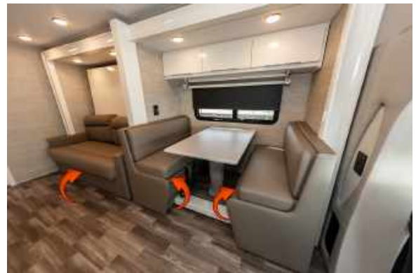
Figure 59.4 Depending on Model, Table Leg(s) and Top(s) May Be Stored Under Sitting Cushions as Noted with Red Arrows. Note: These Areas Also Provide For Additional Storage.
