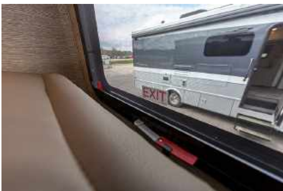
Figure 118.3 Emergency Exit Window Closed
