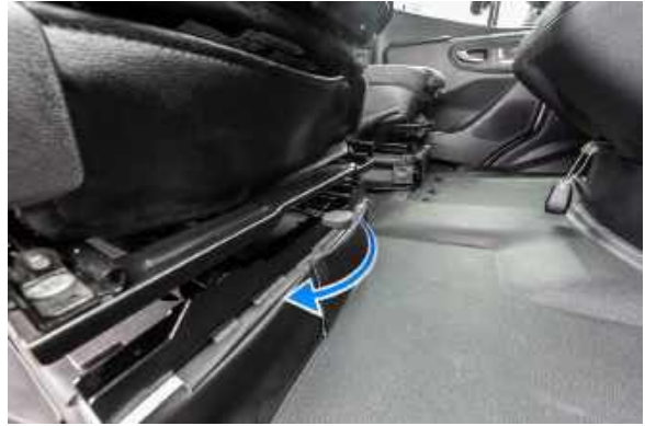
Figure 65.2 To Rotate Seats, Push Release Lever Towards Door and Start Rotating the Seat Inwards
