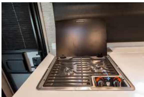
Figure 44.3 Push In and Turn Burner Knobs Clockwise and Hit Ignitor Button to Light. Turn Burner Knobs Counter Clockwise to Turn Off
