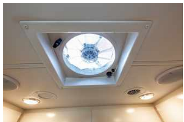
Figure 120.1 Overhead Vent Fan
