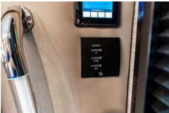
Figure 119.3 Awning Control Switch
