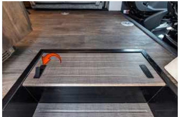
Figure 76.2 Coach Battery Compartment, to Unlock Press On the Rear Most Tab to Release the Locking Mechanism
