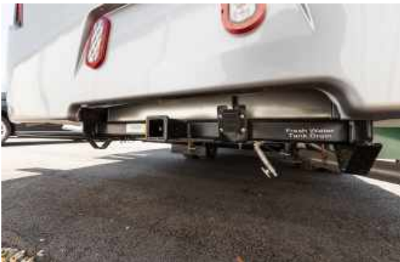
Figure 30.1 Towing Hitch and 7 Way Pin Connector
