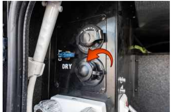
Figure 107.1 City Water Intake Marked with Red Arrow and Blue Handle Turned to City
