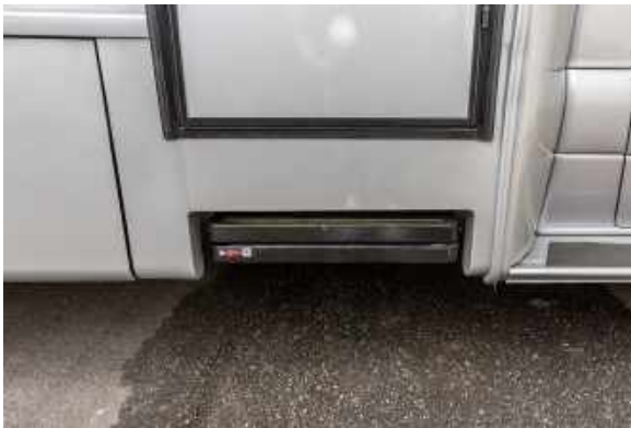
Figure 98.1 Side Entry Exterior Power Steps in Retracted Position
