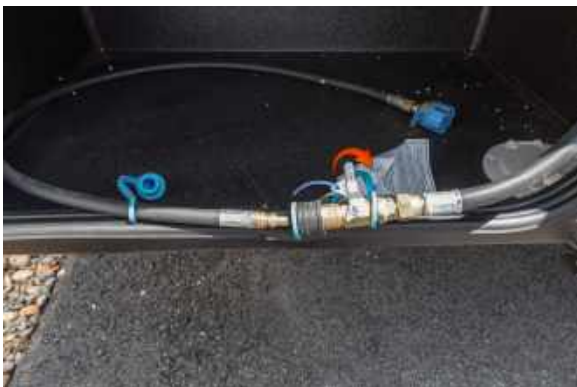
Figure 40.1 Propane Quick Connect With Valve Lock in Open Position
