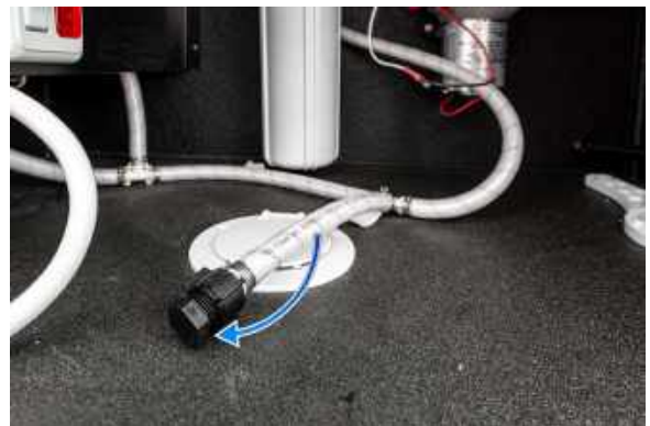
Figure 107.2 Remove Plug Marked with Blue Arrow to Insert Winterization Hose
