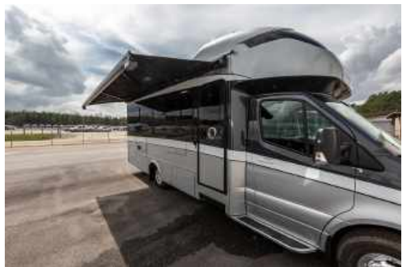
Figure 119.2 Power Awning In Extended Position
