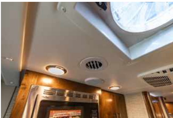
Figure 102.2 Ceiling Area with Lights and Vent Fixtures Shown
