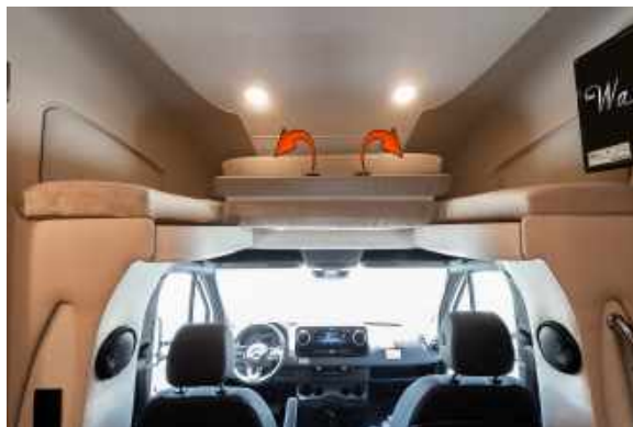
Figure 66.2 To Create Over Cabin Bunk Bed Pull the 2 Metal Handles Towards the Rear of the Motorhome
