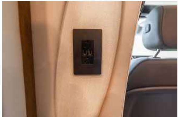
Figure 79.1 120V VAC Receptacle with USB Ports
