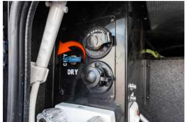
Figure 109.2 To Use Water From the Fresh Water Tank, Turn Blue Valve to "DRY"
