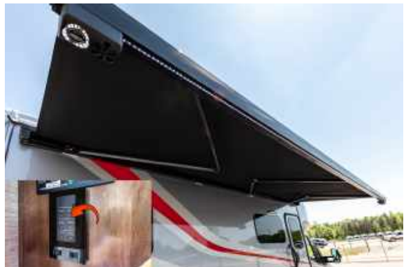
Figure 119.4 Awning LED Lighting with Light Control Panel Shown
