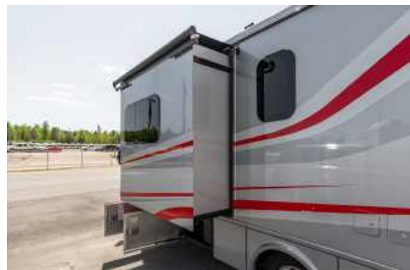
Figure 64.4 Slide-Out Room Extended
