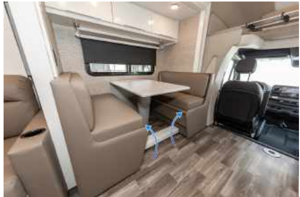
Figure 62.2 Dinette Booth. Lift Up Bottom Seat Bases to Reveal Storage Area and Seat Belts
