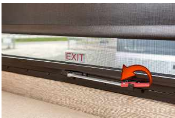
Figure 28.3 Lift Red Handle and Move Towards Left To Extend
