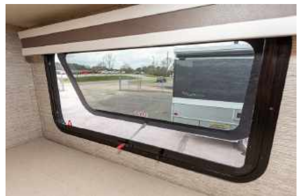
Figure 118.4 Emergency Exit Window Handle Engaged
