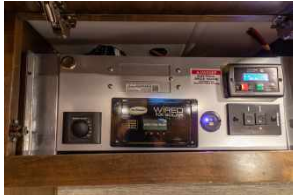
Figure 47.2 Truma Water Heater Control Switch on Master Panel Located in Bedroom of Coach
