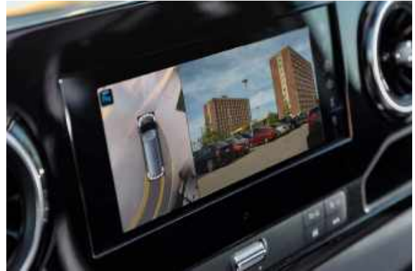
Figure 123.1 Mercedes Benz Sprinter Rear View Camera On In Dash Radio
