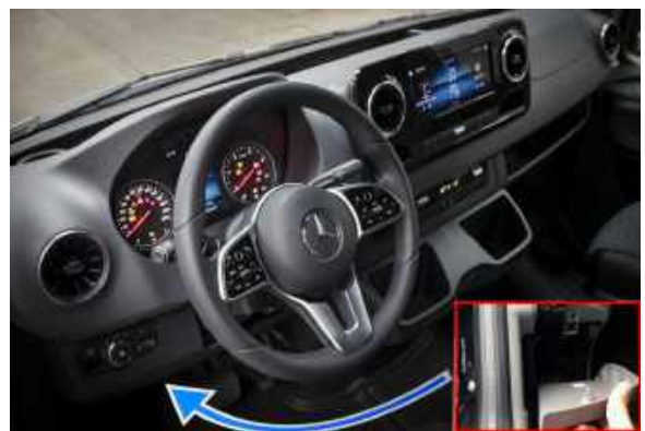
Figure 84.2 Chassis Fuse Panel Location Under Dash
