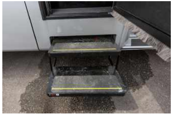
Figure 98.2 Side Entry Exterior Power Steps in Extended Position
