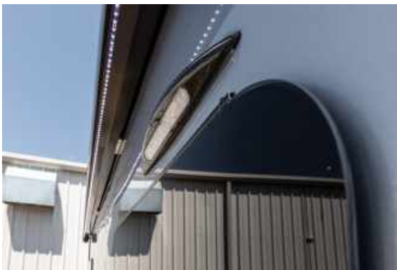
Figure 97.1 Exterior Security/Patio Light
