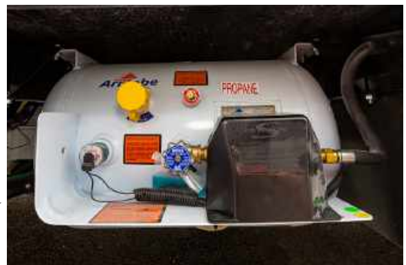
Figure 17.1 LP Propane Gas Tank
