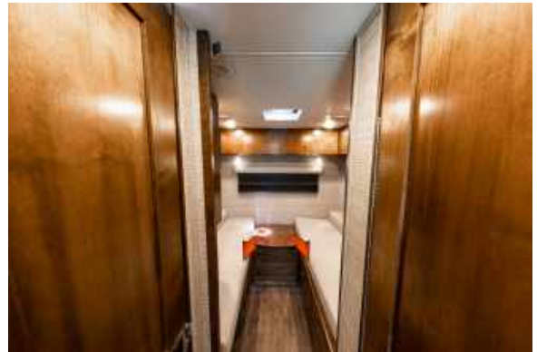
Figure 68.2 To Convert To King Bed, Pull the Center Support From Its Stored Position and Pull Towards Front of Motorhome
