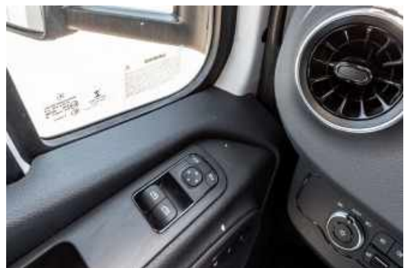
Figure 100.2 Sprinter Multi Directional Mirror Control and Mirror Selector
