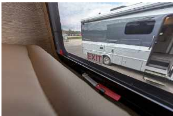
Figure 28.1 Emergency Exit Window in Living Area
