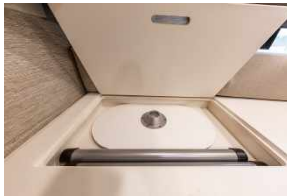
Figure 67.4 Depending on Model Remove Passenger Side Bed Cushion to Reveal Extra Storage or Table Top and Table Leg Storage
