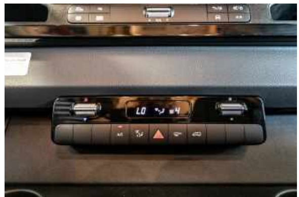
Figure 123.2 Mercedes Benz Sprinter Cooling/Heating Dashboard Controls
