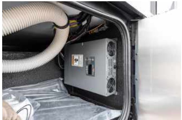
Figure 81.1 Inverter; Located In Outer Storage Compartment on Passenger Side of Motorhome
