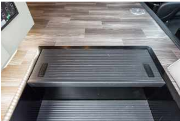
Figure 76.1 Coach Battery Compartment Locked
