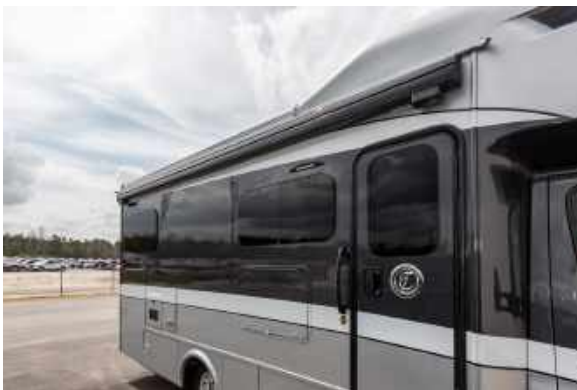
Figure 119.1 Power Awning In Closed Position
