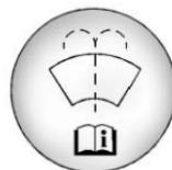
Open the cap with the washer symbol on it. Add washer fluid until the tank is full. See *Engine Compartment Overview* ▷ 218 for reservoir location.
