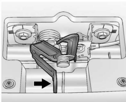
2. Go to the front of the vehicle and move the secondary hood release lever toward the right side of the vehicle.
