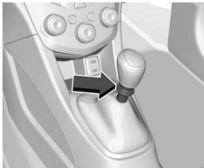
**R (Reverse)** : To back up, press down the clutch pedal, lift up the reverse lockout ring on the shift
