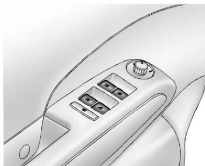
If equipped, the power windows work when the ignition is on, in ACC/ACCESSORY, or when Retained Accessory Power (RAP) is active. See *Retained Accessory Power (RAP)* ▷ 187.
