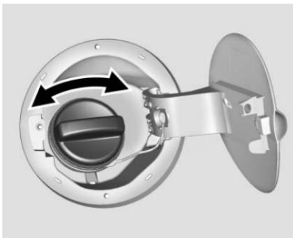
The fuel cap is behind a hinged fuel door on the passenger side of the vehicle.
