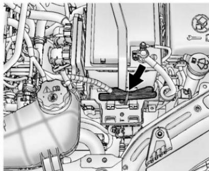
2. Open the hood and unwrap the electrical cord. The cord is located in the driver side of the engine compartment, near the battery. It is shipped from the factory with a tie holding it in place. Use care in removing the tie so that the cord is not damaged.
