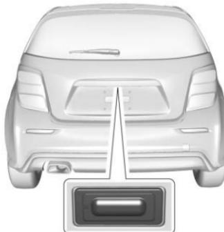
To open the liftgate from the outside, press
