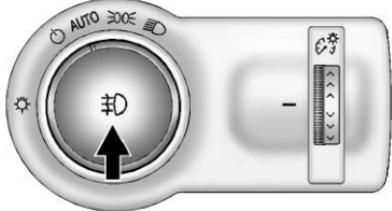
If equipped with front fog lamps, the button is on the outboard side of the instrument panel.
