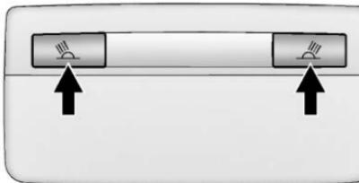
For vehicles with front reading lamps, they are in the overhead console.
