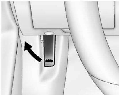
1. Pull the hood release handle inside the vehicle. It is located on the lower left side of the instrument panel.
