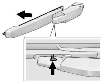
3. Once the blade pin disengages from the wiper arm, remove the wiper blade by sliding the pin out of the guide hole.
