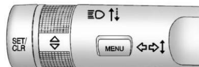
**⊖** : Push the turn signal lever away from you to turn the high beams on.
