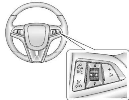
Some audio steering wheel controls could differ depending on the vehicle's options. Some audio controls can be adjusted at the steering wheel.
