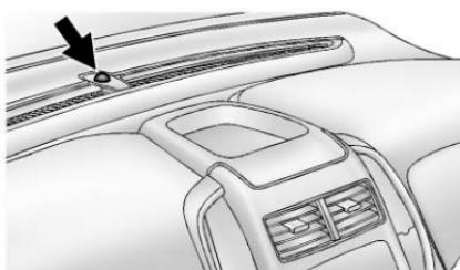
The vehicle has a light sensor on top of the instrument panel. Make sure it is not covered, or the headlamps will be on when they are not needed.
