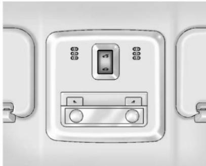
If equipped, the sunroof only operates when the ignition is on or Retained Accessory Power (RAP) is active. See *Retained Accessory Power (RAP)* ▷ 187.
