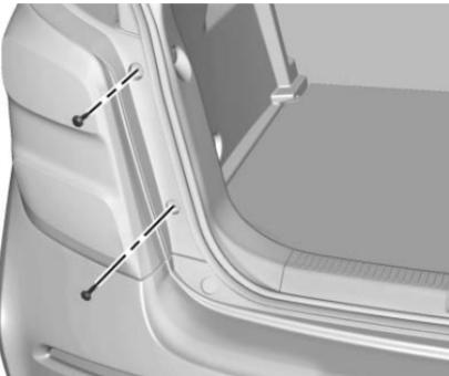
2. Remove the two screws, which secure the taillamp assembly.
