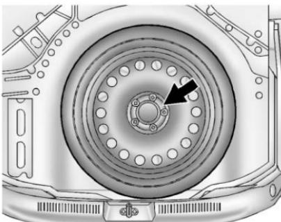
3. Turn the retainer counterclockwise and remove it from the compact spare.
