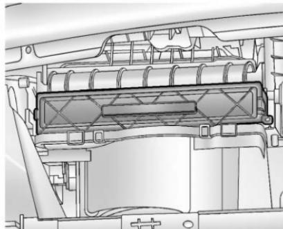
1. Open the glove box completely and disconnect the damper on the outboard side.
