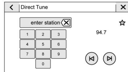
Access Direct Tune by touching the Tune screen icon on the AM, FM, or SXM screen to bring up the keypad. Navigate up and down through all frequencies using  $\triangleleft$  or  $\triangleright$ . Directly enter a station using the keypad. When a new station is entered, the information about that station displays on the right side. This information will update with each new valid frequency tuned to.
