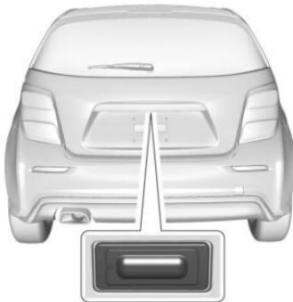
To open the liftgate from the outside, press
