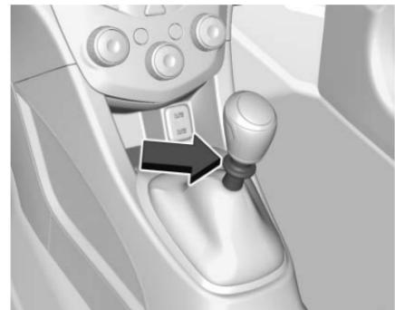
The manual transmission is equipped with a reverse lockout ring. To shift into R (Reverse), press down on the clutch pedal, lift up the ring on the shift lever, and shift into R (Reverse). Let up on the clutch pedal slowly while pressing the accelerator pedal.
