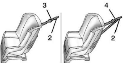
A top tether (3,4) is used to secure the top of the child restraint to the vehicle. A top tether anchor is built into the vehicle. The top tether attachment hook (2) on the child restraint connects to the top tether anchor in the vehicle in order to reduce the forward movement and rotation of the child restraint during driving or in a crash.
