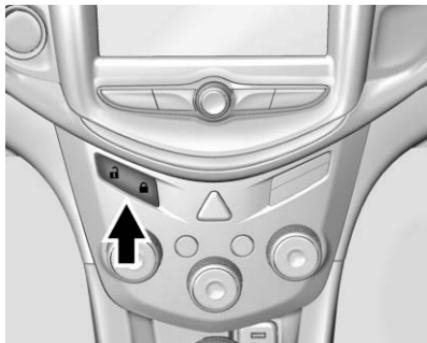
To lock the doors from inside the vehicle:
