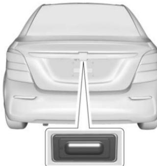
To open the trunk from outside of the vehicle:
