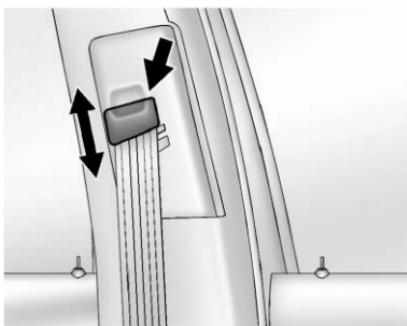
The adjuster can be moved up by pushing the slide/trim up. To move the adjuster down, press the release button and move it down.
