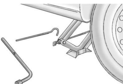
5. Insert the jack handle into the jack and the wheel wrench onto the end of the jack handle.
