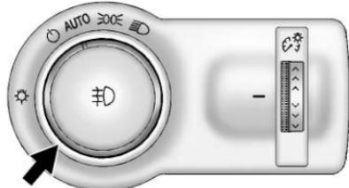
The exterior lamp control is on the instrument panel to the outboard side of the steering column.
