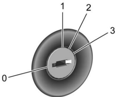
The ignition switch has four different positions.
