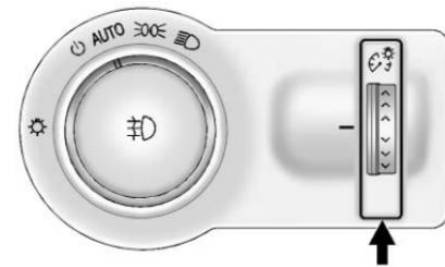
This feature controls the brightness of the instrument panel controls and infotainment display screen. The thumbwheel is to the left of the steering column on the instrument panel.
