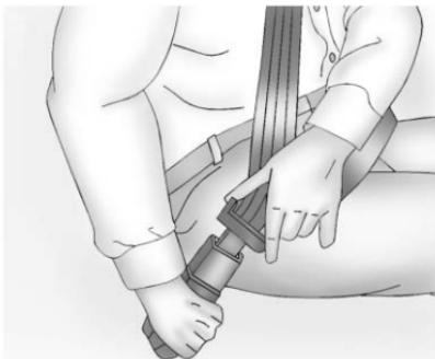
3. Push the latch plate into the buckle until it clicks. Pull up on the latch plate to make sure it is secure. If the belt is not long enough, see *Seat Belt Extender* 66. Position the release button on the buckle so that the seat belt could be quickly unbuckled if necessary.
