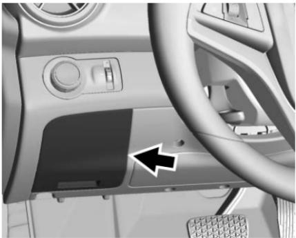
The instrument panel fuse block is on the underside of the driver side instrument panel.
