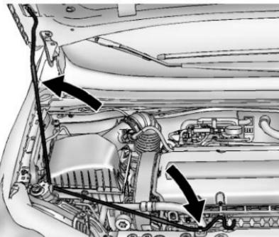
3. Lift the hood and release the hood prop from its retainer, located in front of the engine compartment. Securely place the hood prop into the slot on the underside of the hood.
