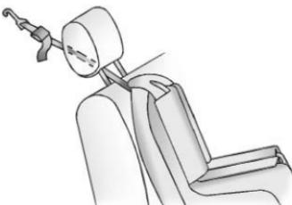
If the position you are using has an adjustable headrest or head restraint and you are using a single tether, raise the
