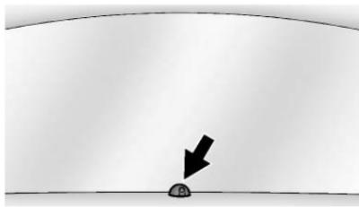
The indicator light on the instrument panel near the windshield indicates the status of the system.
