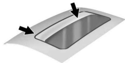
Dirt and debris may collect on the sunroof seal or in the track. This could cause an issue with sunroof operation or noise. It could also plug the water drainage system. Periodically open the sunroof and remove any obstacles or loose debris. Wipe the sunroof seal and
