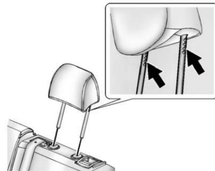
1. Insert the head restraint posts into the holes in the top of the seatback. The notches on the posts must face the driver side of the vehicle.
