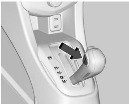
2. Press the + (plus) end of the button on the side of the shift lever to upshift, or press the - (minus) end of the button to downshift.
