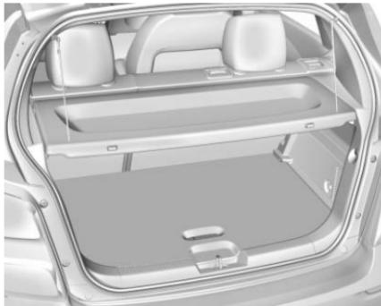
The load compartment cover can be used to conceal objects under it, or it can be removed and placed on the bottom of the load compartment to carry larger loads.
