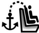
To assist in locating the top tether anchors, the top tether anchor symbol is on the cover for sedan models or near the anchors on hatchback models.
