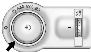
The exterior lamp control is on the instrument panel to the outboard side of the steering column.
