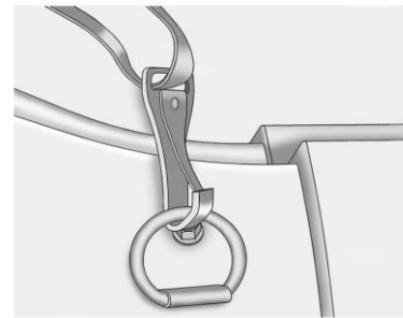
4. Attach one end of the strap to a cargo tie-down in the rear of the vehicle.
