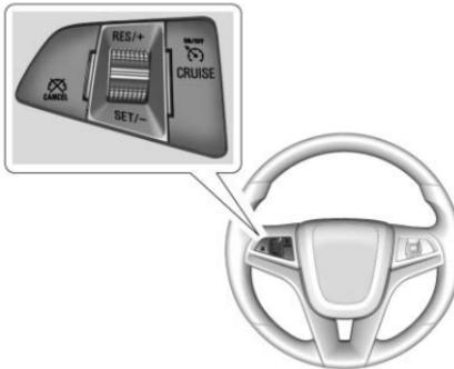
CRUISE : Press to turn the cruise control system on and off. A white indicator comes on in the instrument cluster when cruise is turned on.
