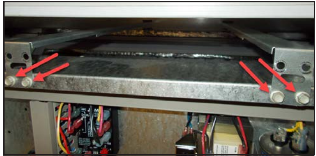
FIGURE 6 Remove Four Screws
