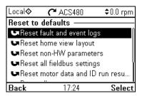
The **Reset to defaults** submenu enables you to reset parameters and other settings.
