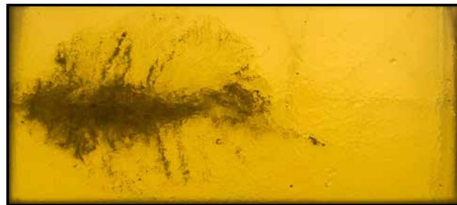
Gel block test illustrates how the Ballistic Tip® Lead Free patented Fragmenting Copper Core™ technology results in complete fragmentation within the first 2 inches of penetration.
