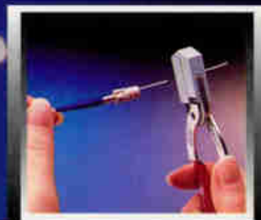
Step 3: Strip the 900 \mu\text{m} buffer. Clean the bare fiber with an alcohol wipe.
