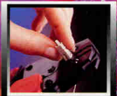
Step 9: Using the crimp tool, apply an additional crimp to the ferrule assembly to further secure the fiber.
