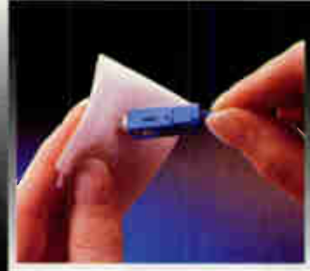
Step 11: Clean the connector with high-grade isopropyl alcohol and lint-free wipes. This step removes any fragments or dirt remaining on the fiber.
