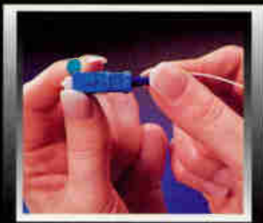
Step 10: Slide the boot into place over the rear of the connector assembly. Push the blue shroud over the front of the white housing.
