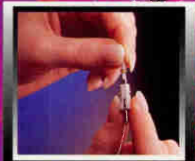
Step 8: Align the key of the inner housing with the key of the ferrule. Push the ferrule into the housing until it snaps into place.
