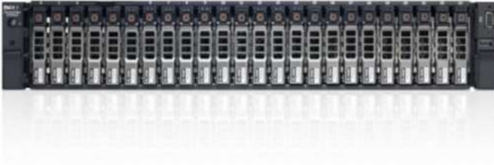
Figure 4. R720xd front view (2.5-inch chassis without bezel)
