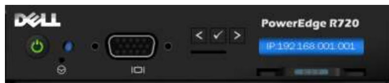
Figure 9. R720 LCD control panel
