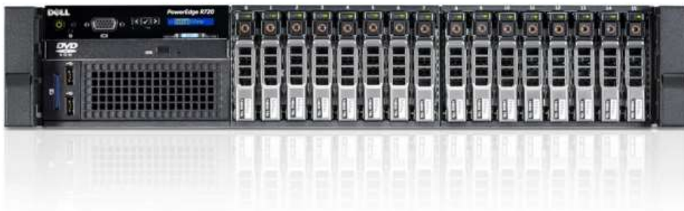
Figure 2. R720 front view (2.5" chassis without bezel)
