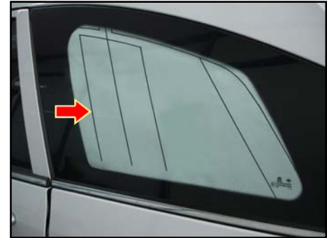
Antenna located on third quarter glass
