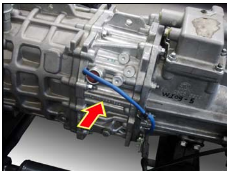
Gear Box Number - Punched
