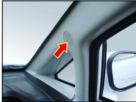
Tweeter located on 'A' pillar
