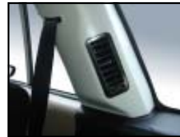
A.C. air vents on 'C' pillar for third row seat
