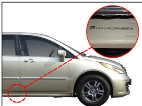
Chassis No. - Punched on RH Long member
