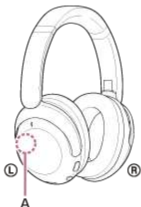
A: Location of the built-in antenna
