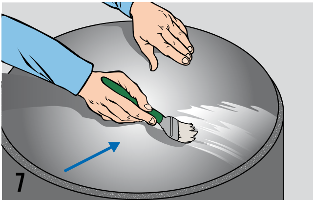
...and the top of the tank with K-FLEX® Contact Adhesive.
