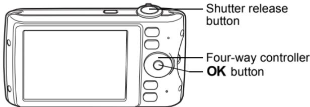
**1** Press the four-way controller (▼) in **REC** mode.
