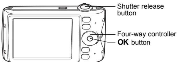
1 Press the four-way controller (▼) in **◀▶** mode.
