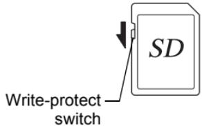
**SD** appears on the display when the card is write-protected.
