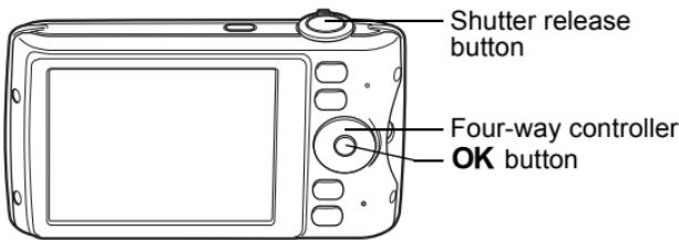
**1 Press the four-way controller (▼) in
