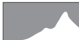
When the image is too dark, the part to the left is cut off (dark portions) and when the image is too bright, the part to the right is cut off (bright portions).
