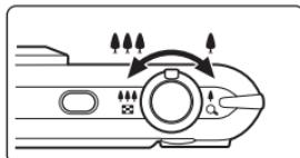
When you continue to turn to the right (↑), the camera automatically switches from optical zoom to Intelligent Zoom.
