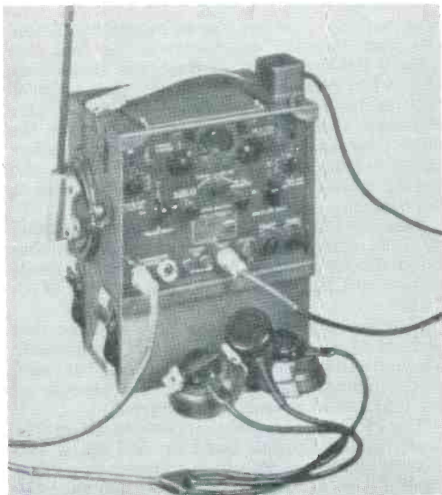
Beautiful but a bomb, the famous TBY, a 27 mc/s Navy transceiver. With its super-regen receiver and drifting transmitter, it was the disaster of the age.
