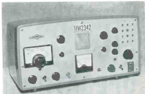
Just to show what can be done with military surplus, here's the result of converting a Navy MBF rig (made by Collins) to CB use. The rig is owned by Frank Webster, KKX4717 (ex-11W2342), of Hollywood, Calif. Original frequency range was 60 to 80 mc/s, and this was the major task, the cabinet was also custom made by Frank. The rig is as slick as a greased ground plane and the envy of all who see it (and what a fantastic signal too).
