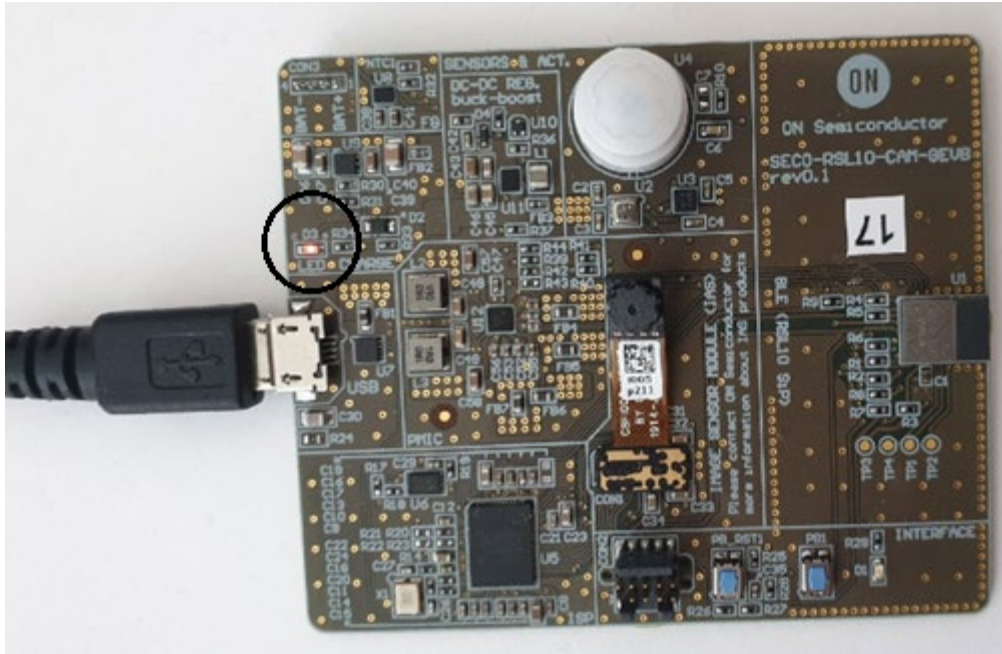
Fig.7 LED D3 continuously blinks (fault operation, FAN54120 didn't start properly). Make sure plugging the USB cable once unplugged, happen after at least 10s to allow Battery charger controller start properly.
