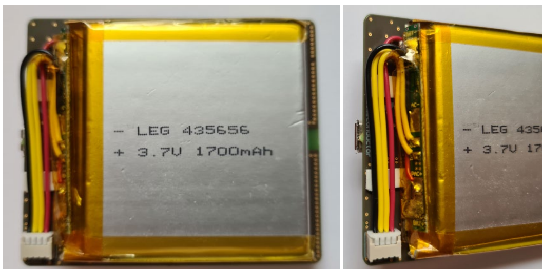
Fig.12 Physical implementation of the battery and its protection circuit from bottom side of SECO-RSL10-CAM-GEVB
