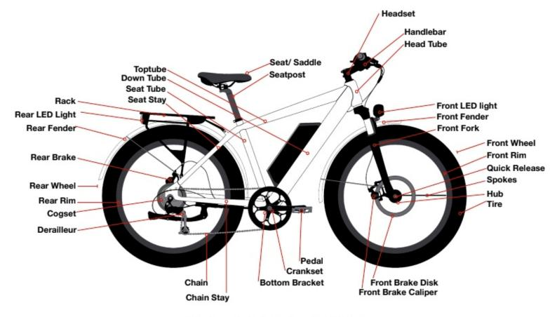
Note: Side with chain is Drive side / Right side Side without chain is Non Drive side / Left side
