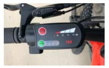
**Note**: Before mounting the bike to ride, hold the brake lever. It cuts off the main power to the bike. It is always safest to mount the bike before turning on the bike, as turning it on enables the throttle. If
