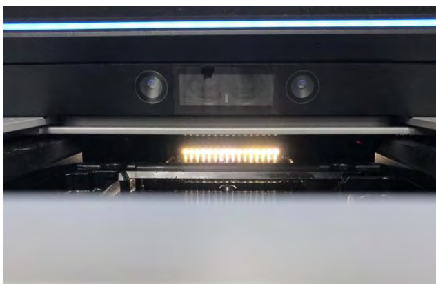
Figure 5.4: Optical mating surface in the Alto instrument from the cartridge view.
