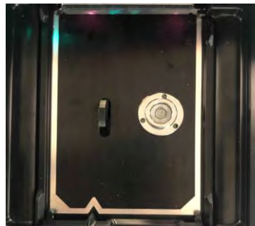
Figure 4.7: Setting up bubble level in the cartridge loading bay.
