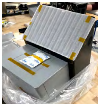
Figure 4.4: Remove the tapes from the Alto once the device is set up on a lab bench.
