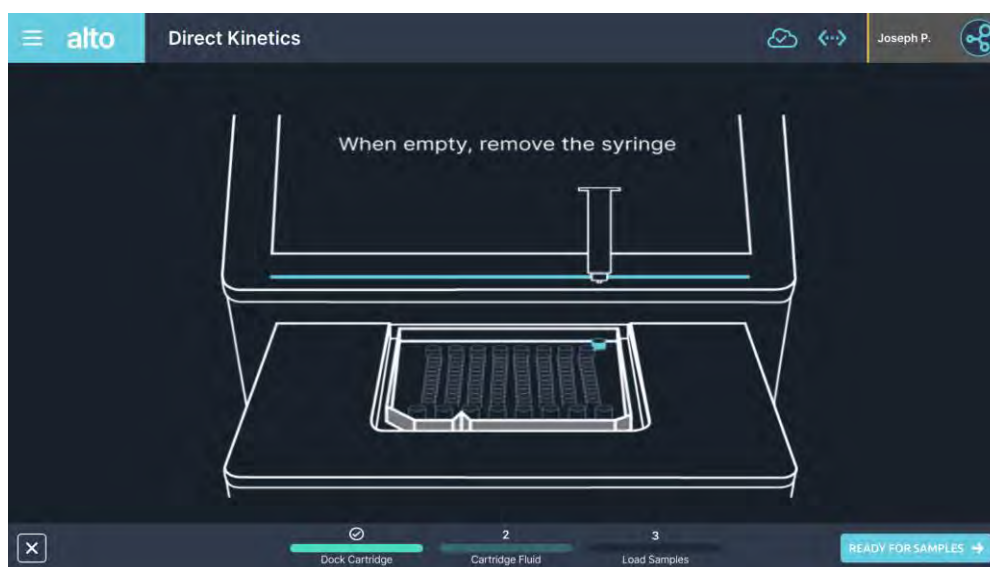
Figure 5.30: Remove the empty cartridge fluid syringe from the cartridge.
