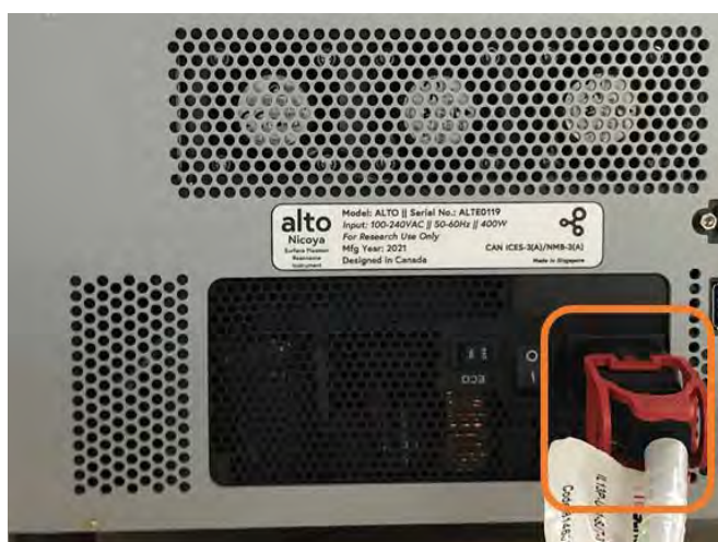
Figure 4.17: Securing the power cable into the IEC power inlet.
