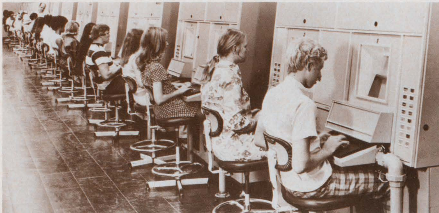
Operators read addresses on envelopes passing through windows in front of them and punch out an extraction code on a keyboard. A computer translates this to a bar code that allows machines to route the letters from then on.
