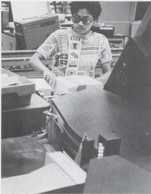
Optical character reader (OCR), Model I, in New York City's Church Street Post Office, reads 43,200 printed and typed letter envelopes an hour.
