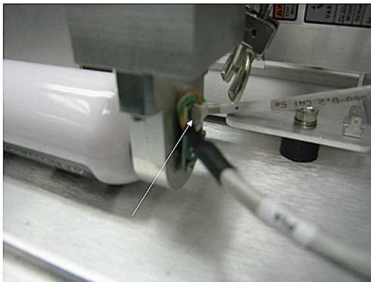
Figure 3: Cable to Calibrated Leak Connection
