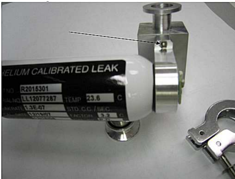
Figure 4: Calibrated Leak Screws
