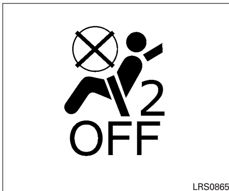
Front passenger air bag and status light
