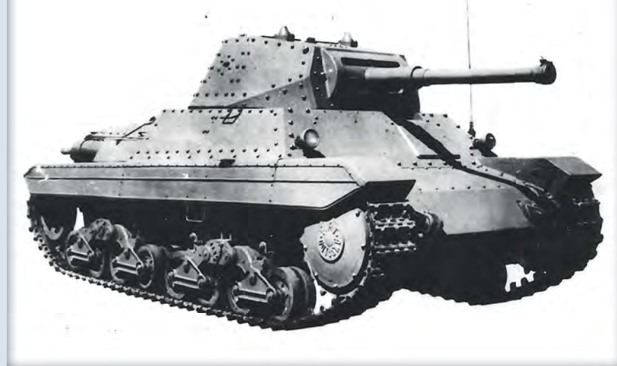
ABOVE: Despite a more powerful engine and better gun the M15/42 looks a lot like its predecessors BELOW: A P26/40 viewed from the front, sloped armour makes it look impressive but it wasn't very thick by infantry tank standards and the method of construction was going out of favour
