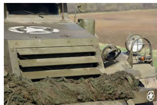
ABOVE AND BELOW: Engine armour open and closed - .25in thick panels protect the engine and radiator, they can be closed from inside the cab, but the engine can't run for long with them closed without overheating
