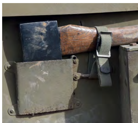
Pioneer tools were carried on each side below the cab doors, the half-track is amply fitted with externally accessible lockers, racks, boxes and hooks
