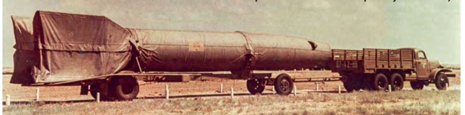
BELOW: An R-2 rocket being towed by a 6x6 ZiS-151 truck at the Kapustin Yar polygon. The standard production ZiS-151 dates the photograph as the very early 1950s rather than late 1940s (early production ZiS-151s produced from 1948 had a partially wooden cab)
