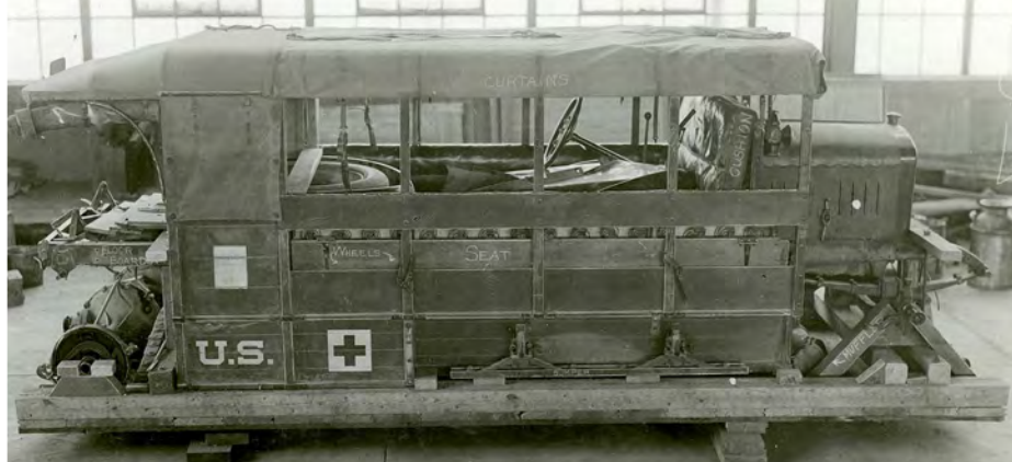
ABOVE: A new GMC ambulance having been crated for delivery to France. Interestingly the whole chassis has been loaded inside the body to best utilise space
