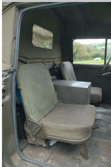
Roger replaced all the canvas in the M715 and had a new battery box fabricated
