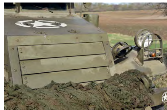
ABOVE AND BELOW: Engine armour open and closed - .25in thick panels protect the engine and radiator, they can be closed from inside the cab, but the engine can't run for long with them closed without overheating
