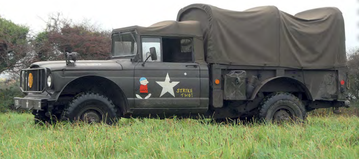
ABOVE: Roger found that the chassis was sound with some welding required only to sills and the floor pan at the rear of the cab BELOW: Approximately 33,000 made between 1967 and 1969 and had nine years in service but few remain
