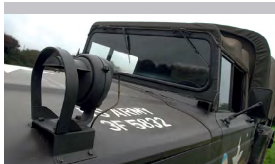
The militarised cab includes a folding windscreen, a feature on other smaller military Jeeps plus removable canvas roof
