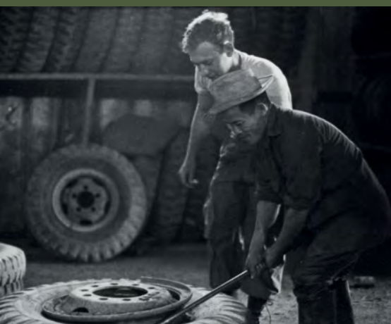
The 1st Force Service Regiment deployed a large number of trucks to deliver such as food, fuel, water and ammunition to marines deployed in the field. Maintenance personnel had to deal with an average of 50 punctured tyres every day. Here we see Corporal Raymond T Bruton on December 23, 1968, training a Vietnamese civilian employee on how to deal with a punctured tyre (CORPORAL JOHN S KRILL / 26393781)
