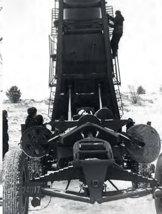
ABOVE LEFT: The Soviet successor to the V-2 in firing position on the Russian steppe, without protection from the elements ABOVE RIGHT: The 8U24 transporter-erector trailer for the R-1 was a basic assembly intended for limited distance travel only. Note the conventional truck-type leaf-spring for shock absorption
