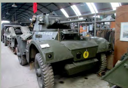
1942 Daimler Mk1 Armoured Car. Armed with a 2 Pdr main gun and Besa machine gun, this vehicle was used in the film A Bridge Too Far
