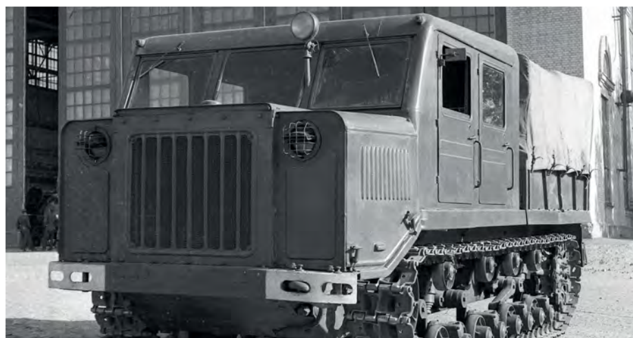
ABOVE: The AT-S medium artillery tractor was developed to replace the wartime Ya-12 and post-war M-2. The vehicle could accommodate a six-man gun or rocket crew in addition to the driver
