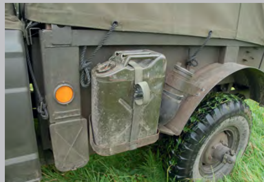
Roger has added a US-specification fuel Jerrycan and petrol filler while behind the rear fender pioneer tools would be fixed to the pick-up body
