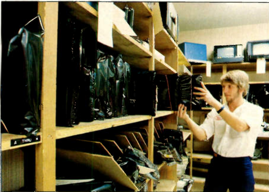
During inventory and shipping, precautions, such as the use of static-shielding bags, can protect electronic devices and circuit boards from ESD damage.
