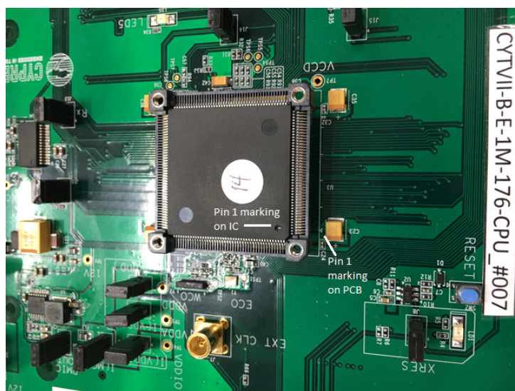
Figure 3-1. Orientation of Device when Inserted in Socket
